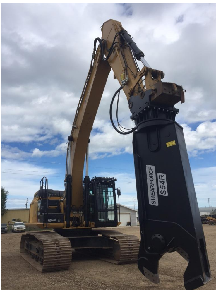
A shearing attachment on an excavator to assist in demolition projects
