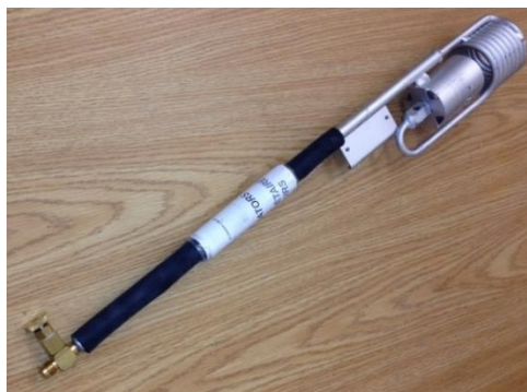
Liquid Propane Torch (note coil tubing on tip for liquid vaporization)
