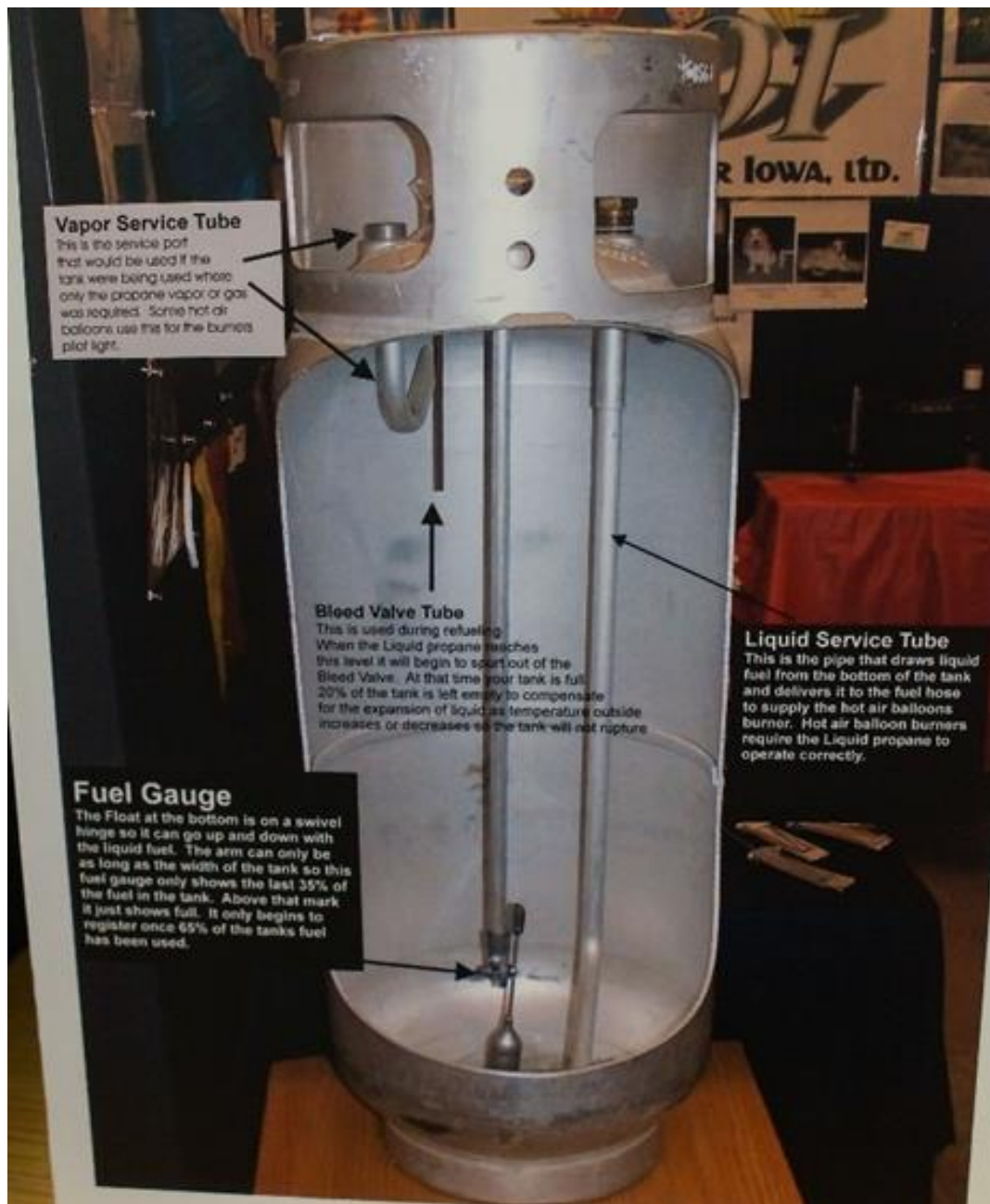
Propane cylinder cut out that shows both the liquid and vapor service tubes.
