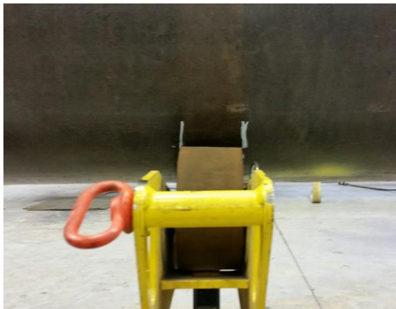
Mark the Stand Position on the Pipe
