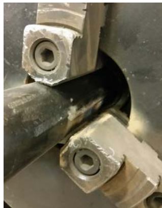
Pipe Inside the Chuck
