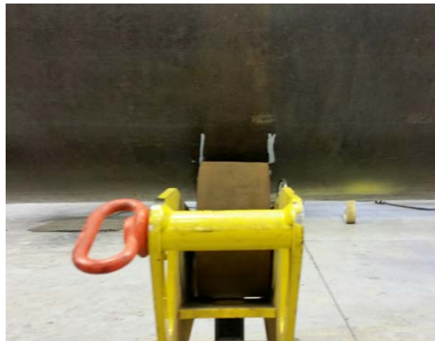
Mark the Stand Position on the Pipe
