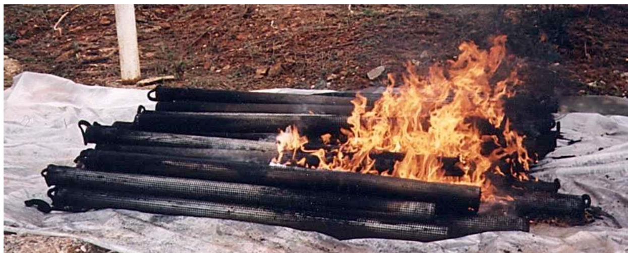
Example of dry filters spontaneously combusting
