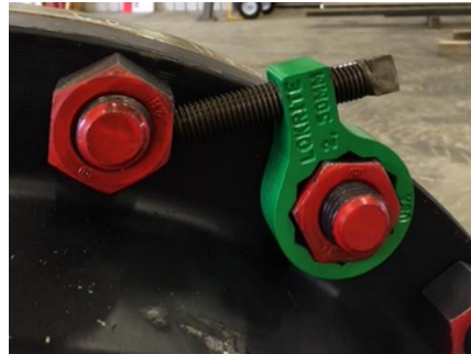
Example of a Hands-Free Backing Tool
