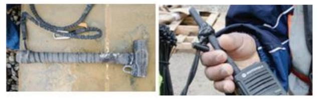
\*\*Note: Tools must not be modified for lanyards unless permitted under OEM\*\*
