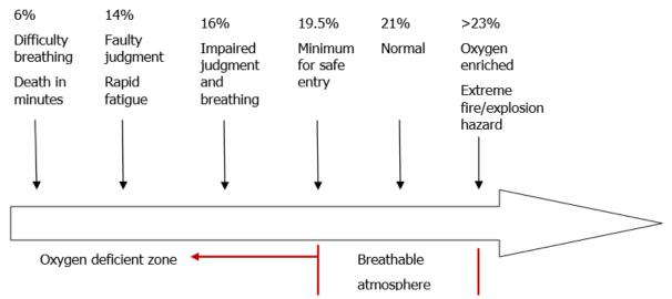
If the oxygen concentration exceeds 23%, the space is oxygen-enriched, which increases the likelihood of fires or explosions by increasing the likelihood of ignition of flammable material, as well as the rate of reaction. Oxygen enrichment may occur from leaking gases, welding equipment.
