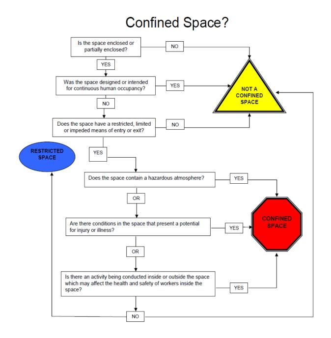
Although OH&S does not specify different levels of confined space, the OSSA RCOP does. There are three levels which reflect the degree of hazard, as well as the lowest hazard level, which is a restricted space. These four classifications are detailed below. Although required only on OSSA-governed sites, these classifications provide useful guidance for managing confined spaces.
