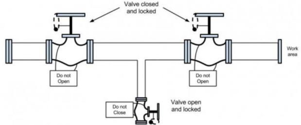
Any isolation performed with respect to confined space entry should be performed in conjunction with CPES's Lock Out-Tag Out (LOTO) code of practice (COP-05), and only by competent workers.
