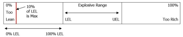
All gases have an explosive range with a Lower Explosive Limit (LEL) and an Upper Explosive Limit (UEL). When the fuel and air mixture is below the LEL or above the UEL, ignition will not occur.
