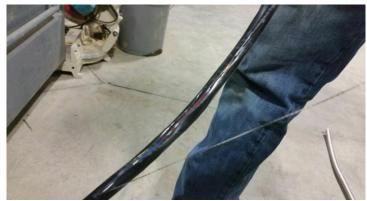
**DO** Check the wire to identify any damage to the insulation.
