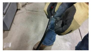
**DO** Pull the string down the cable to expose the inner cables.
