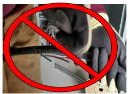
**DON'T** Count on a non-cut proof gloves to protect you from lacerations. Typical leather gloves are not intended to offer protection from knives. Remember that all gloves are considered a last line of defense and no glove can be protect you all the time.
