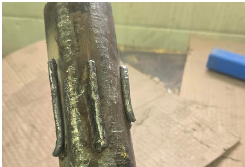
Welds directly on the jig can help keep it from spinning in the chuck
