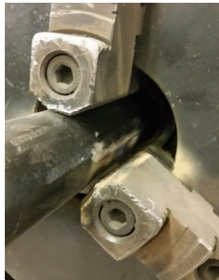
Pipe Inside the Chuck
