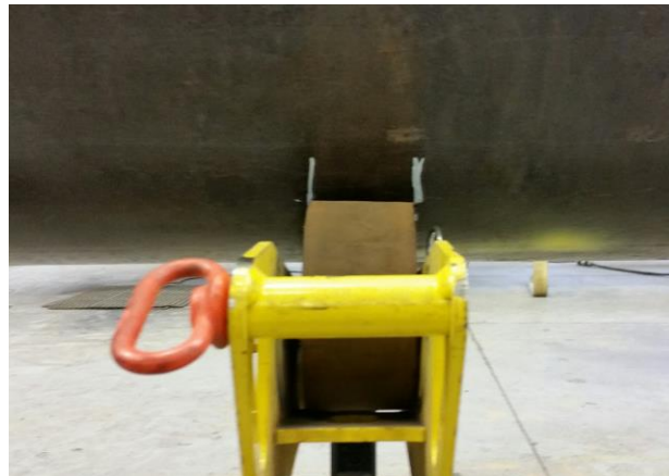
Mark the Stand Position on the Pipe
