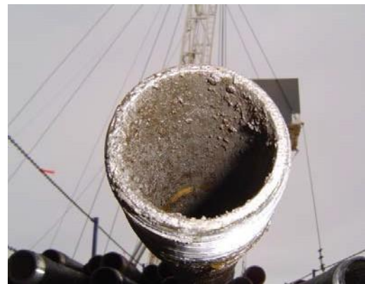
Scale containing NORM on service line
